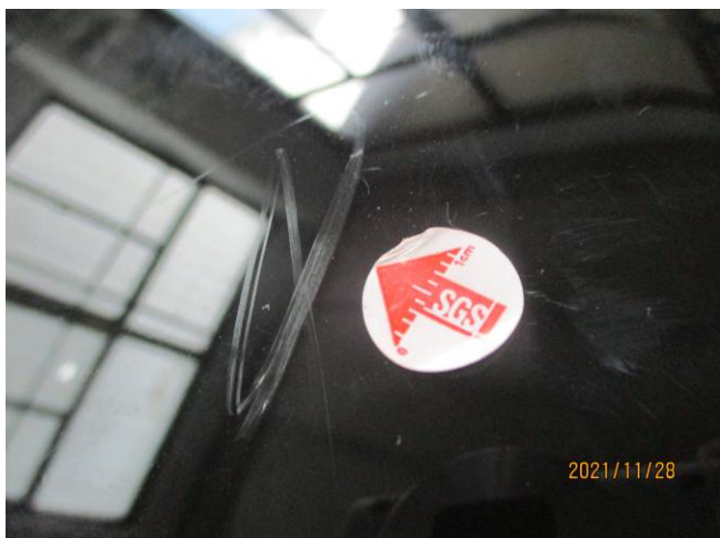
LF-012B defect-Scratch mark on unit (2)
