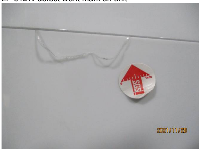
LF-012W defect-Plastic film on unit
