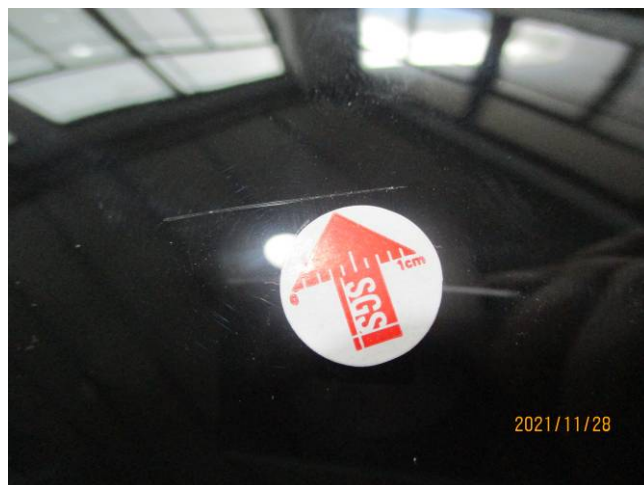
LF-012B defect-Scratch mark on unit (3)
