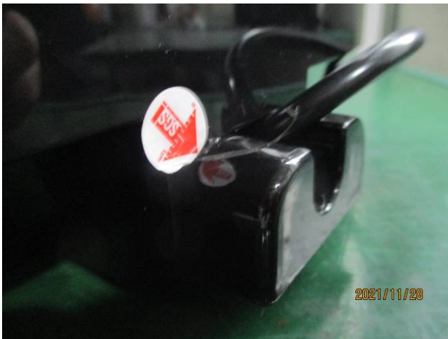
LF-012B defect-Flash on unit
